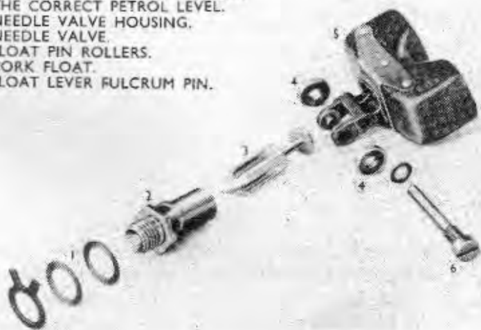
Needle valve, housing and float assembly.
