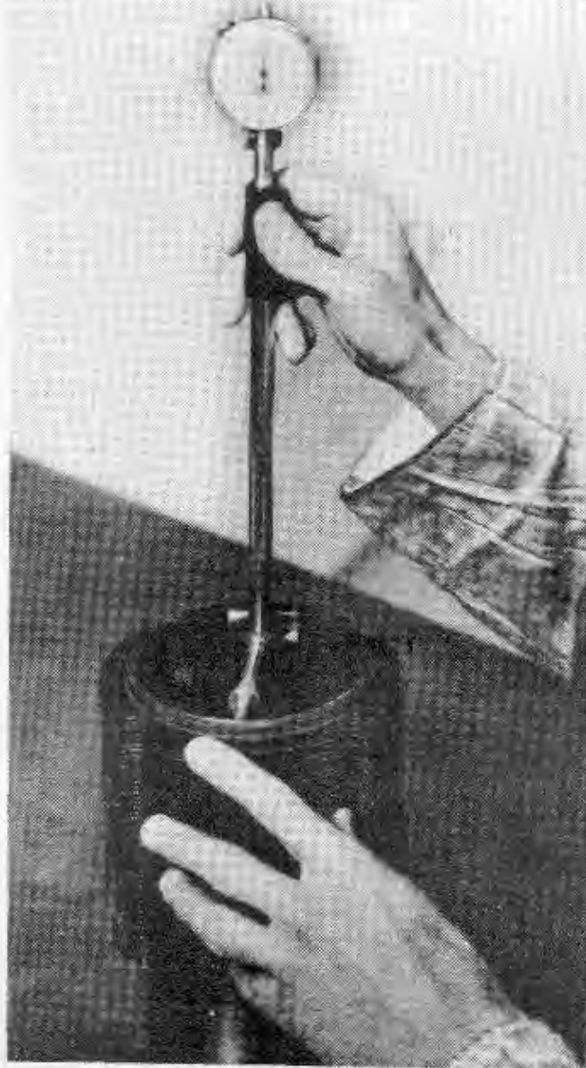
Fig. 8. Checking cylinder barrel for wear
