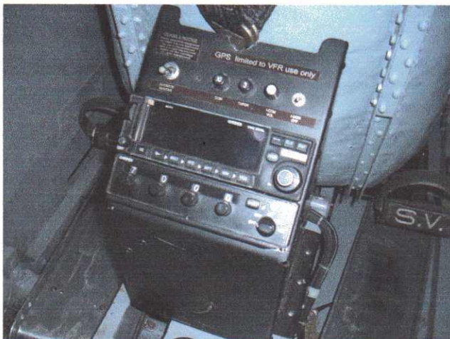
Radio, GPS and transponder set behind the front seat. Well away from sunlight.
