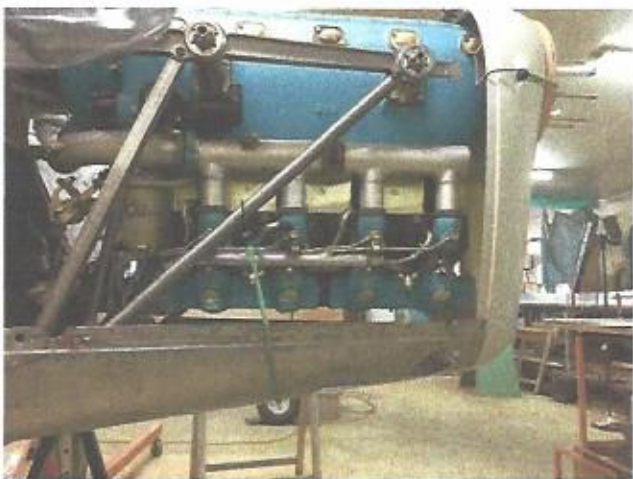
What a big one you've got! A LOM engine being installed by Didier Ferrand in France.
