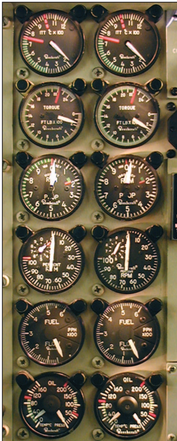
Figure 14-7. Engine instruments—split shaft/free turbine engine.
