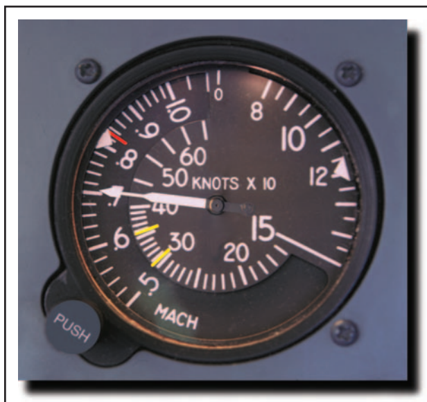
Figure 15-8. Jet airspeed indicator.
