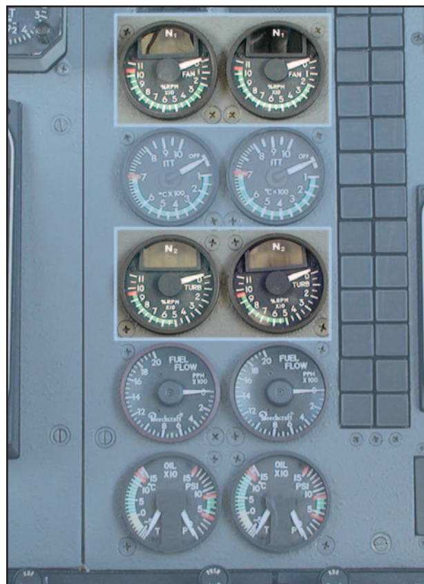
Figure 15-4. Jet engine r.p.m. gauges.
