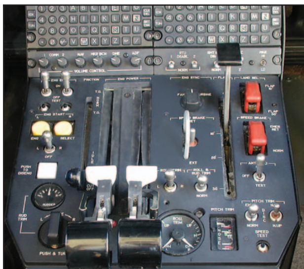
Figure 15-3. Jet engine power controls.
